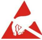
This integrated circuit can be damaged by ESD. UniverChip Corporation recommends that all integrated circuits be handled with appropriate precautions. Failure to observe proper handling and installation procedure can cause damage. ESD damage can range from subtle performance degradation to complete device failure. Precision integrated circuits may be more susceptible to damage because very small parametric changes could cause the device not to meet its published specifications.
